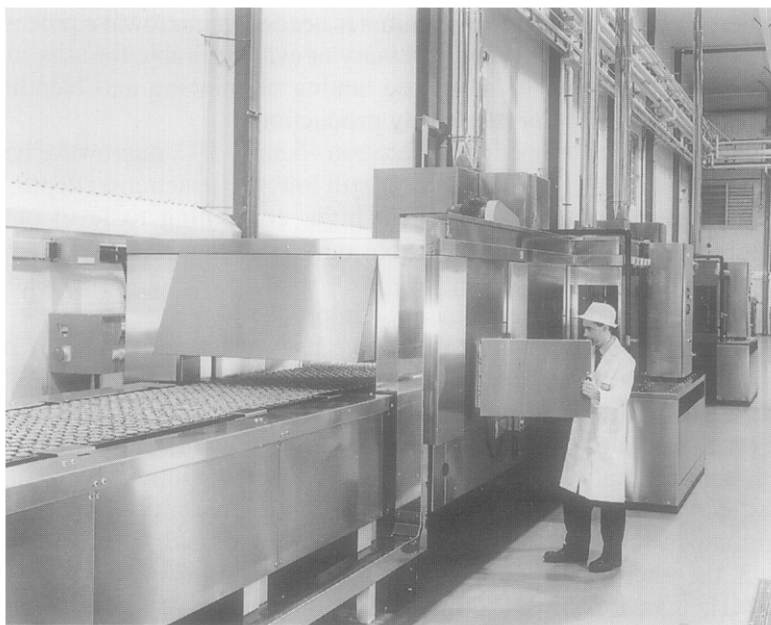
FIG. 26. Microwave-assisted baking oven (APV, 1995).
